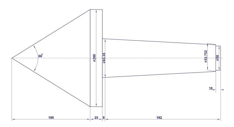
Note: Run - Out of Centre Ground Shall not Exceed 0.05 mm with respect to Taper
