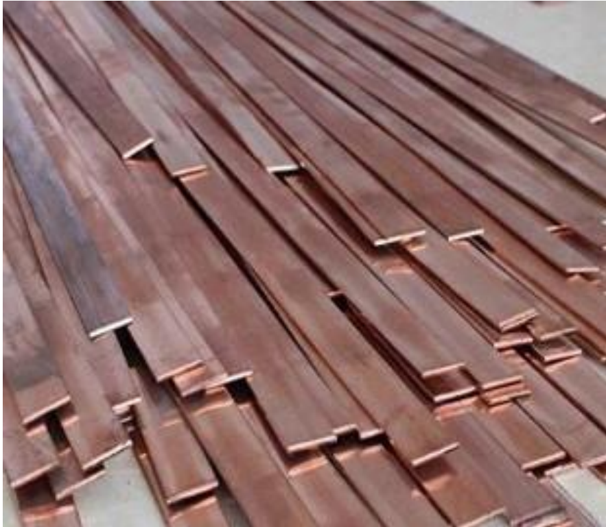
Picture-7 Copper bar, length 16m, width 5cm, Thickness 3mm
