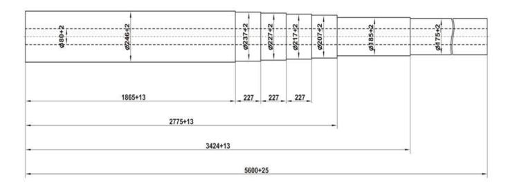
TECH REQUIREMENTS: BENDING OF BORE SHALL NOT EXCEED 3 MM
