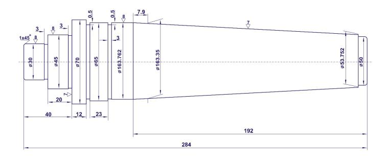
Note: Run - Out of Centre Ground Shall not Exceed 0.05 mm with respect to Taper
